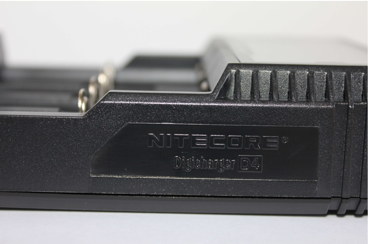
FAKE NITECORE D4 CHARGER – TYPEFACE AND SPACING INCORRECT AND THE FINS ARE ALL THE SAME THICKNESS.
